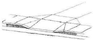
Figure 4-36: Although parallel driveway crossings provide users with level landings, users continuing on the sidewalk are forced to negotiate two ramps.
