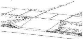
Figure 4-34: On wide sidewalks, there is enough room to provide a ramp for drivers and retain a level landing for pedestrians.
