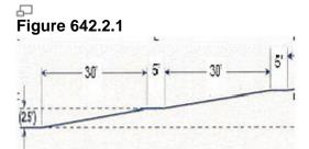
A landing will be located at the top and bottom of all ramps and between segments that have a 30 in. rise. The landing will be at least the width of the ramp with a minimum length of 60 in. If a turn is required the landing must be 5 ft. x 5 ft. For example, a segment with a running slope of 1V:12H, or 8.33% will require a 5 ft. x 5 ft. landing every 30 ft. if it is part of a switchback access route.
